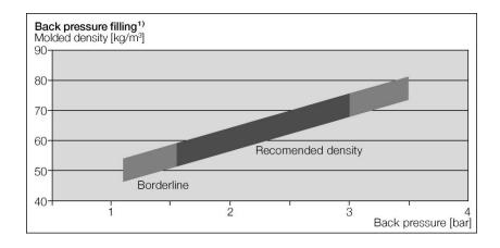
$<sup>^{1)}</sup>$  The Processing data are determined on molded parts (300 x 200 x 60 mm) produced under standard conditions and steam pressure of 3,2 - 3,6 bar. The data apply for average bulk denities.
