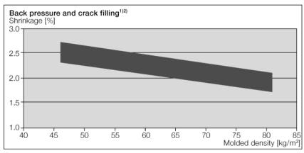
$<sup>^{2)}\,</sup> Shrinkage$  after oven curing (80 °C)
