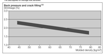
2) Shrinkage after oven curing (80 °C)
